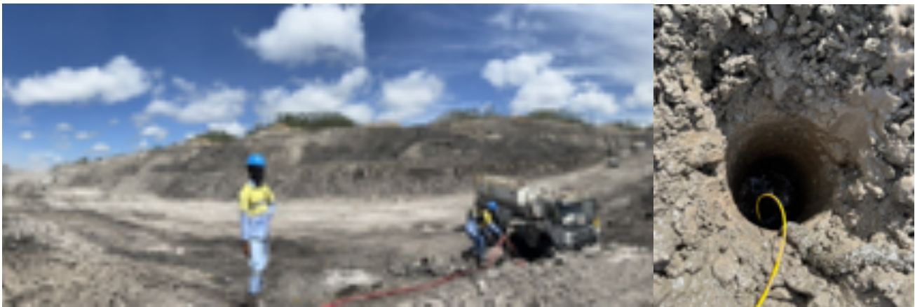
Gambar kegiatan penggunaan solar untuk campuran pada kegiatan blasting di CK MHU Picture of the use of diesel fuel for mixing in blasting activities at CK MHU
